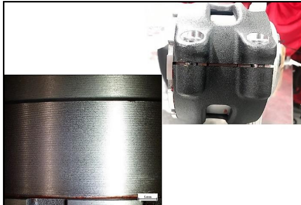
Eccentric hub after tightening the screws to 20Nm
