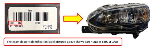
Headlamps with part number 84001FL00B or 84001FL01B will not require replacement. If 84001FL00B or 84001FL01B are found, no replacement is required. Reinstall all removed parts in the reverse order of disassembly.
