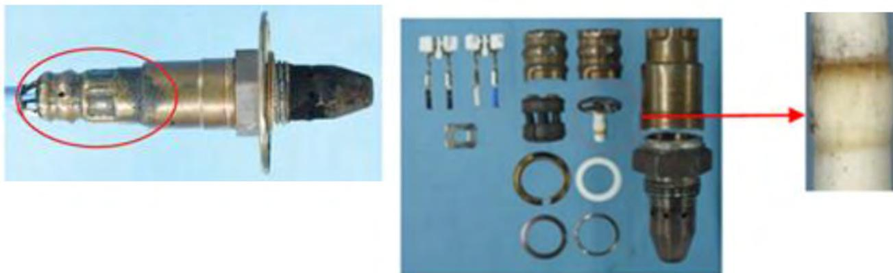
To avoid failure of A/F and O2 sensor and assembly contamination, use the cautions below.
