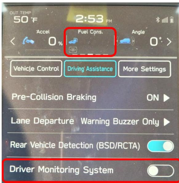
This photo shows the DMS turned off, note the Fuel consumption is blank.
