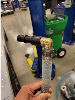
6. Disconnect the two hoses from **the reservoir tank** and connect them to the cleaning equipment as follows:
