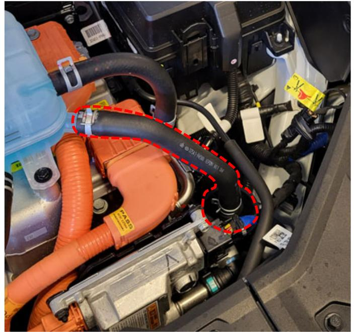
14. Disconnect the two circulation hoses from the reservoir tank hoses and connect them to the air separator hoses as follows:
