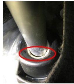
Figure 1. Poor sealing on the intermediate shaft.
