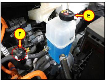
B7. Ensure that the reservoir tank degassing hose valve (F) is closed. If there is no valve, block the flow path as shown in the example to the right.
