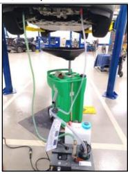
C10. While the cleaning equipment is in operation, remove the reservoir tank to clean the residual coolant and debris inside.
