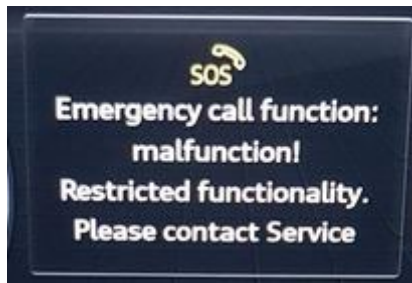
Figure 1. Emergency call malfunction warning.
