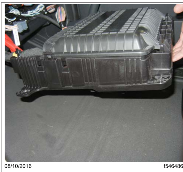
Fig. 11, Lowering the VPDM to the Cab Floor
