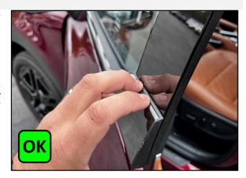
If the outer faceplate <u>is detached or separating from the molding</u> (NG), proceed to the 'Replacement Procedure' below.
