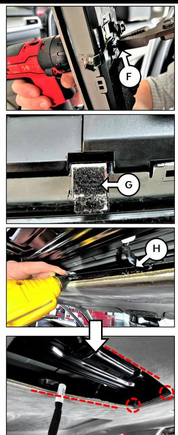
Hot glue application points. Place a bead of hot glue in each corner and/or edge(s) that have detached from the headliner.
