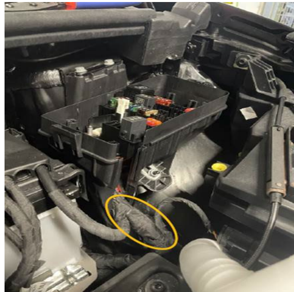
Figure 1: J1 splice point location.
