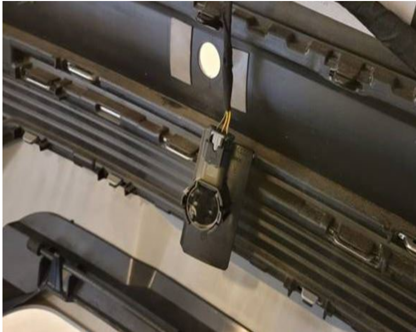
Figure 2: The parking aid mount has come loose.
