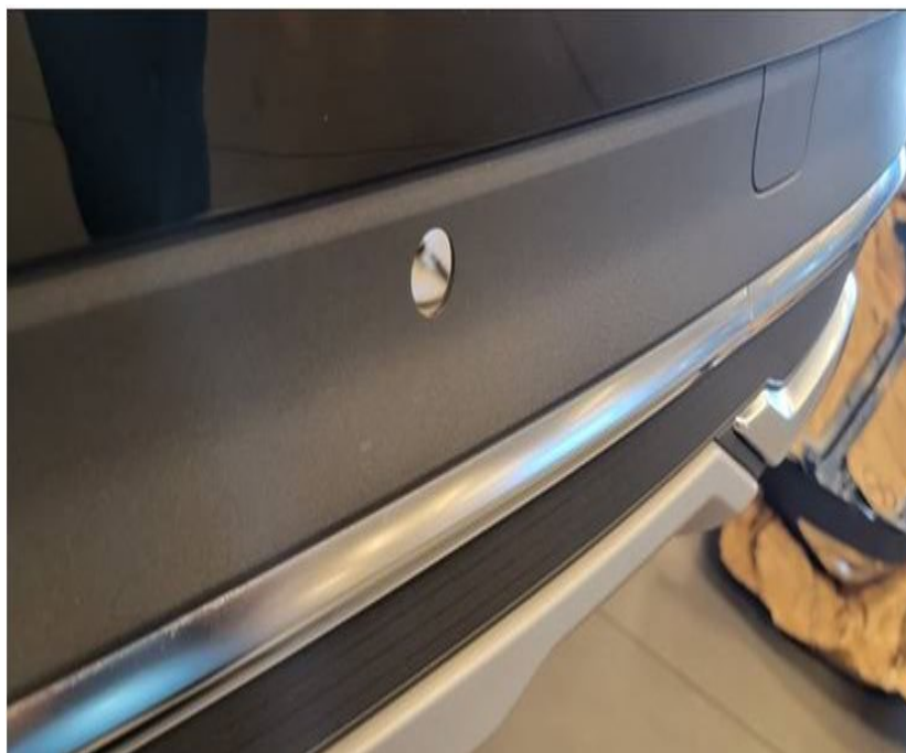
Figure 1: The parking aid mount has come loose.
