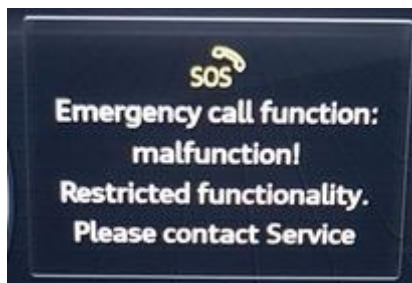
Figure 1. Emergency call malfunction warning.
