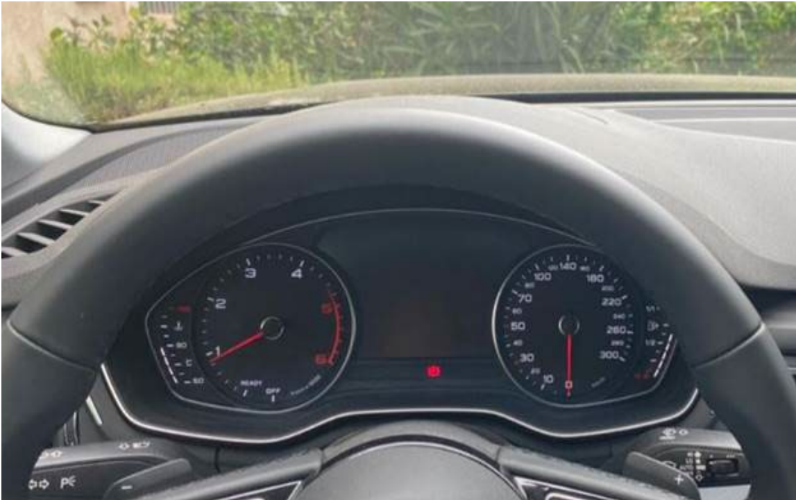
Figure 1. Instrument cluster display is blank.
