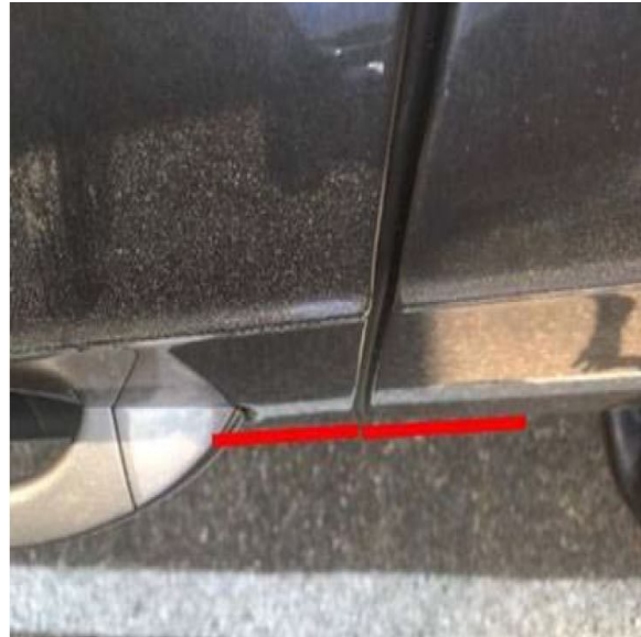
Figure 2. The front door can be flush or slightly under flush to the rear door.
