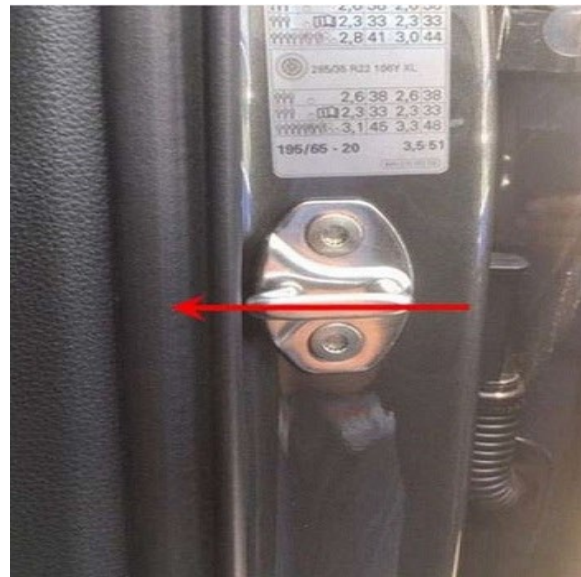
Figure 1. Adjust door striker inward by at least 0.5 mm.
