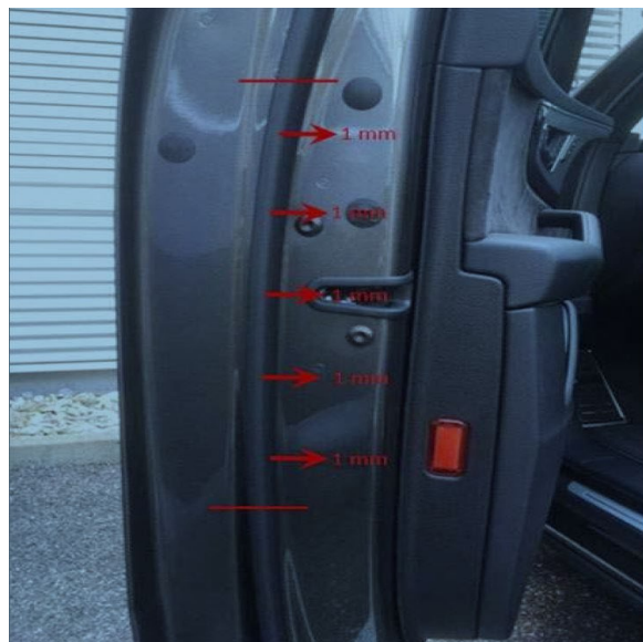
Figure 3. Install the new outer door seal with an inward offset of 1.0 mm.
