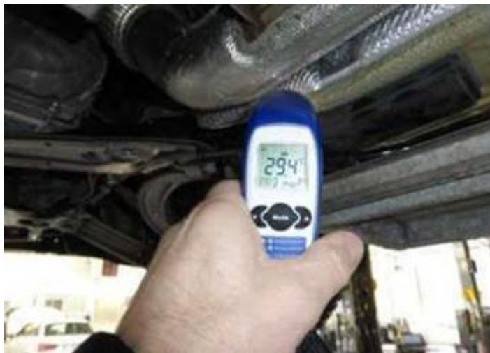
Figure 5. Surface temperature cooled to approximately 30° C (86°F).
