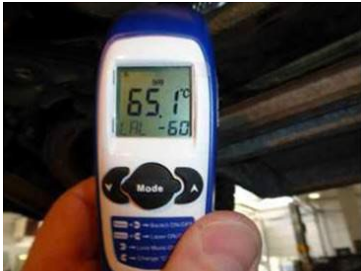
Figure 4. Surface temperature warmed to 65° C (149°F).
