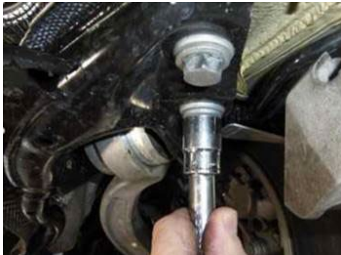
Figure 2. Loosening the front most subframe bolt.
