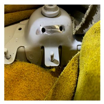
5. Drill a 4.2 mm (approx. 5/32") hole at each end of the indentation/crack to stop any crack propagation.
