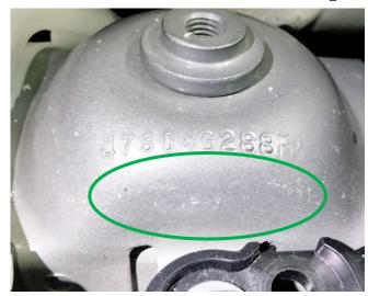
A "good" dome does not show any indications of an indent, nor of a crack/tear.
