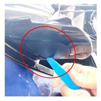
4. Using a fishbone tool, remove the mirror base cap.
