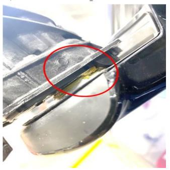
6. Re-grease the bottom metal plates at the pivot point with lubricating grease Kluebersynth LF 44-22.
