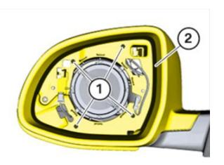
2. Remove the supporting ring by removing the 4 screws.
