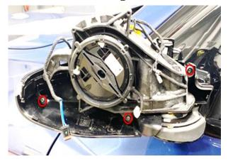
Note: Fold the mirror assembly completely inward to easily remove the lower housing section.
