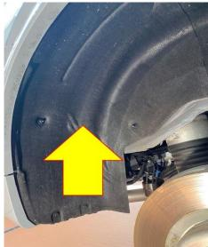
1. Remove the right rear wheelwell cover following the repair instruction listed in ISTA/AIR (51 71 041).
