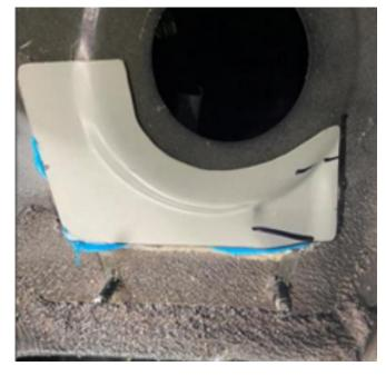
9. Place and press the panel onto the wheelwell hump firmly. Coat the cut edges with K5 adhesive. If necessary, secure the panel using tape to prevent it from slipping off.
