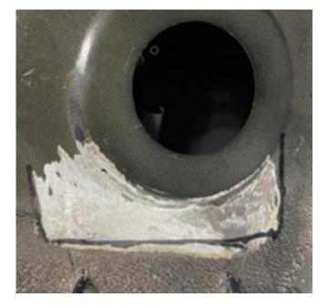
6. Clean the marked area of coating, wax, and body sealant.
