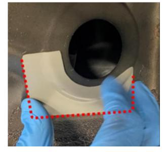
5. Place the cut panel onto the wheelwell hump. Using a marker, trace the panel edges (dotted line) onto the vehicle.
