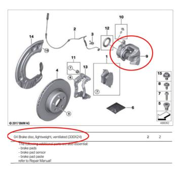
The information of the Service Bulletin only applies to front axle brake disc size of  $330 \times 24$  (4) and calipers with "floating design" (9) as shown.
