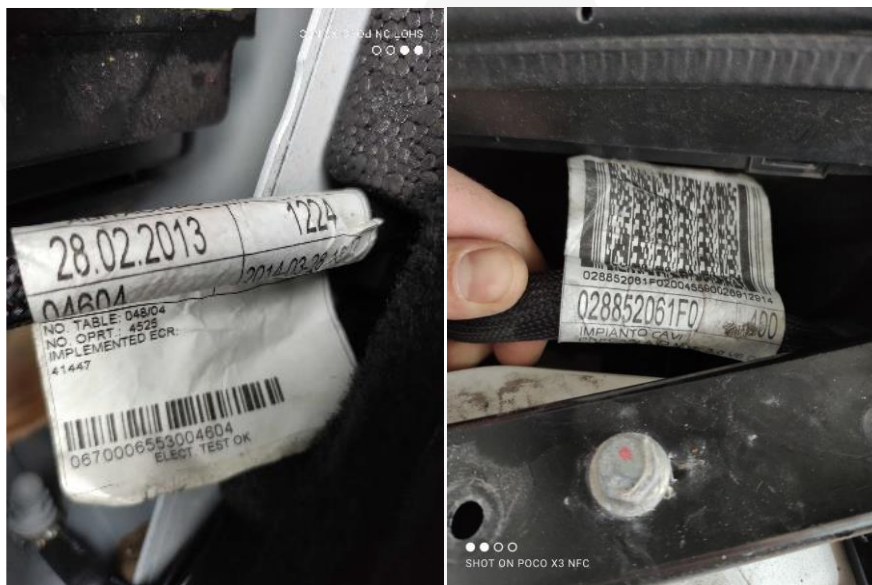
Figure 2: examples of the Traceability Labels of the Battery Positive Wiring (left) and the Recharge Wiring (right).
