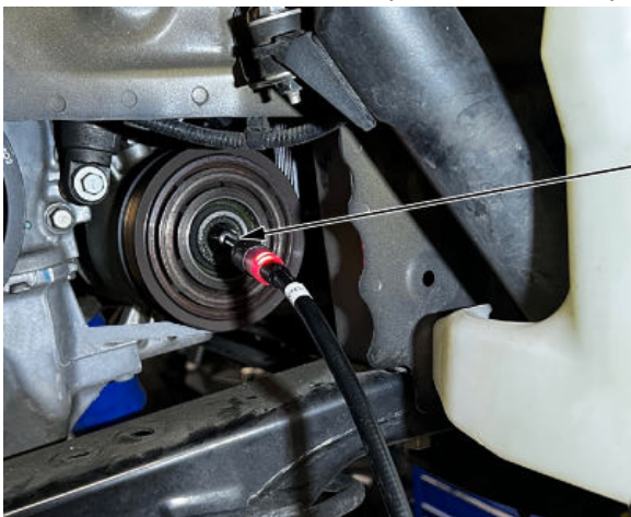
SNOUT OF COMPRESSOR
