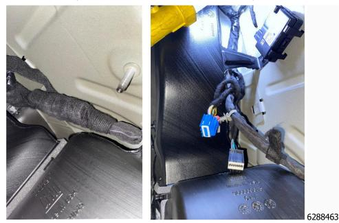
**Note**: The wiring harness for the Parking Assist Control Module may be wrapped around an adjacent wiring harness as shown above. Remove the attaching tape by unwrapping. Do NOT cut the tape as it could damage the wiring harness.
