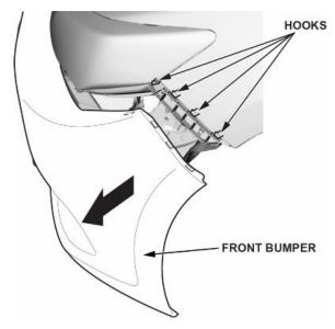
3. With the help of an assistant, while pulling the front bumper away from the side spacer, release the bumper from the hooks on the upper beam.
