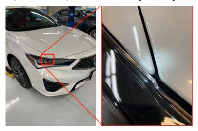
3. There should be clearance between the headlight and the fender as shown below.
