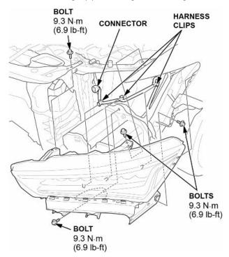
7. Remove corner upper beam from bottom of headlight.
