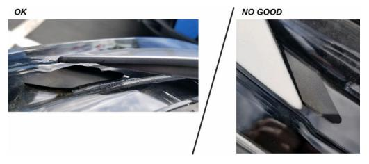
4. If the headlight is contacting the fender, refer to the REPAIR PROCEDURE.
