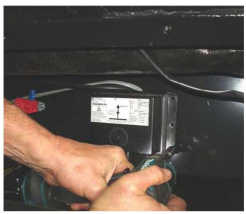
5. The CCM/BSCM is detecting the wrong type of trailer brakes. This is normally caused by an aftermarket device wired into the trailer. The example shown below is an electric over hydraulic-to-electric brake adapter. These adapters are used to make a truck that only works with electric trailer brakes work with a trailer that has electric over hydraulic brakes.
