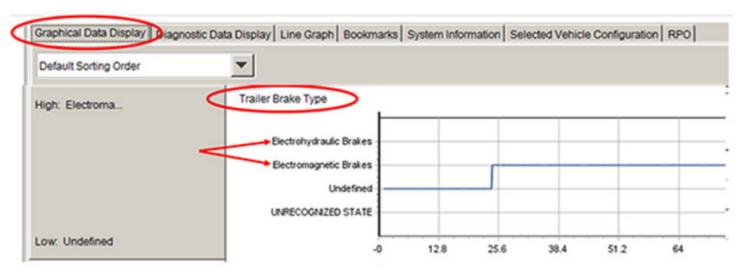
To view "Trailer Brake Control Output Circuit" 47 faults, build GDS2 as follows: CCM/BSCM->Data Display -> parameter "Trailer Brake Control Output Circuit": Okay, Short to Ground, Short to Power, or Unknown. Example, shown below is a trailer with a short to ground on the trailer brake circuit.
