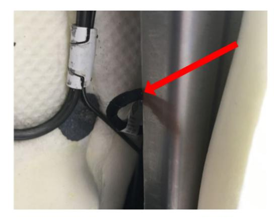
Repair the damaged circuits following the correct procedure in SI for wire and connector repair.
