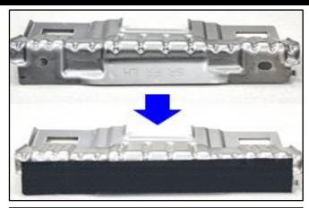
26. Using an awl or Phillips screwdriver, poke a hole in the anti-noise pad through the two (2) mounting holes for both left and right sides.
