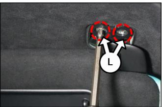
12. Separate the sun visor and detach the connector for both left and right sun visors.
