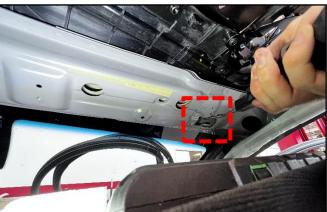
19. Properly tighten all exposed screws, nuts, and bolts along the entirety of the sunroof and roof frame.
