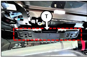
23. Fold over the exposed Tesa® tape and adhere it to the metal mounting clip for both left and right assist handle brackets, as shown.
