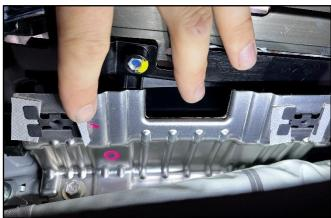
24. Loosen the two (2) assist handle bracket bolts (U) for both left and right sides.
