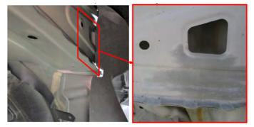
3. The top portion of the padding should be aligned to the reference line of the frame and pasted at the center of the hole. Make sure to paste the L-shaped part (see image below) tightly into the bend of the frame to prevent water from running behind. Paste the bottom half of the padding over and under the edge.
