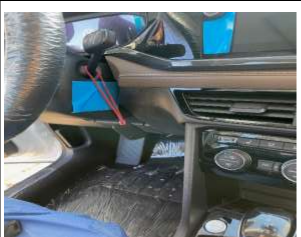
Figure 8. One key tether to the wiper stalk for cars produced in Mexico.
