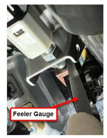
The plunger portion of the switch should extend between the stopper section of the brake pedal and the stop lamp switch threads 1.5mm (0.06 in) in length.
