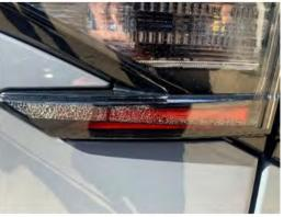
2) If an already warm lamp lens gets cooled down rapidly (e.g. when water is applied to the lens during vehicle washing), a sudden temperature change can occur resulting in the development of condensation.
