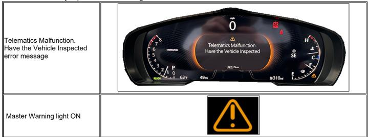
DTC U3000:04 (Telematics communication unit internal malfunction) is stored.
