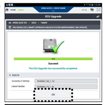
Check if any incidental Diagnostic Trouble Codes (DTC) have been created by the upgrade and clear the DTC(s) present.
