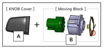
6. Ensure to secure the knob cover (A) using the locking pin shown.
