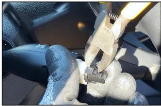
3. Remove the moving block (B) shown on the right.
