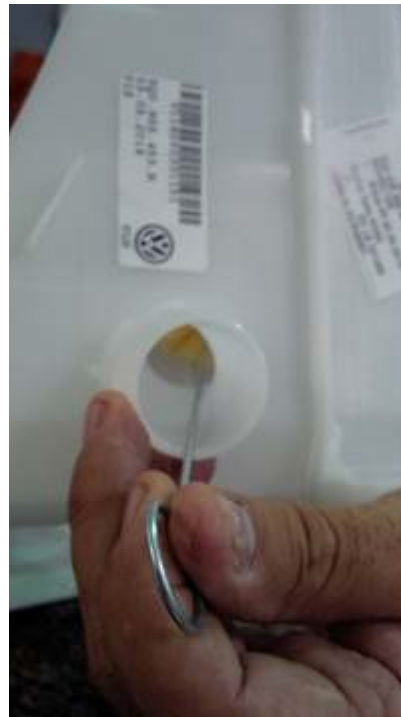
Figure 4. Cleaning the sensor probes.
