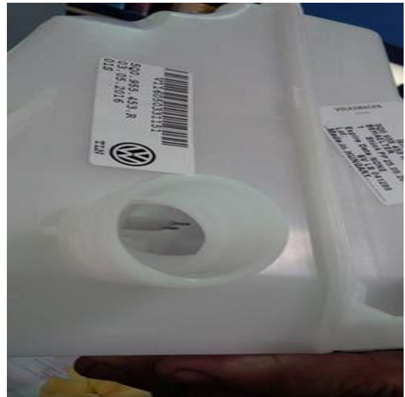
Figure 2. Windshield washer level sensor probes as viewed through the tank opening.
