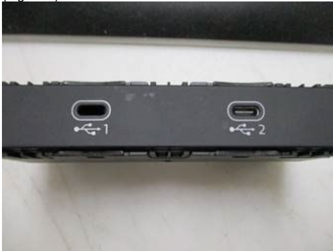
Figure 1: USB socket sheared off the PCB and loose in the housing.
