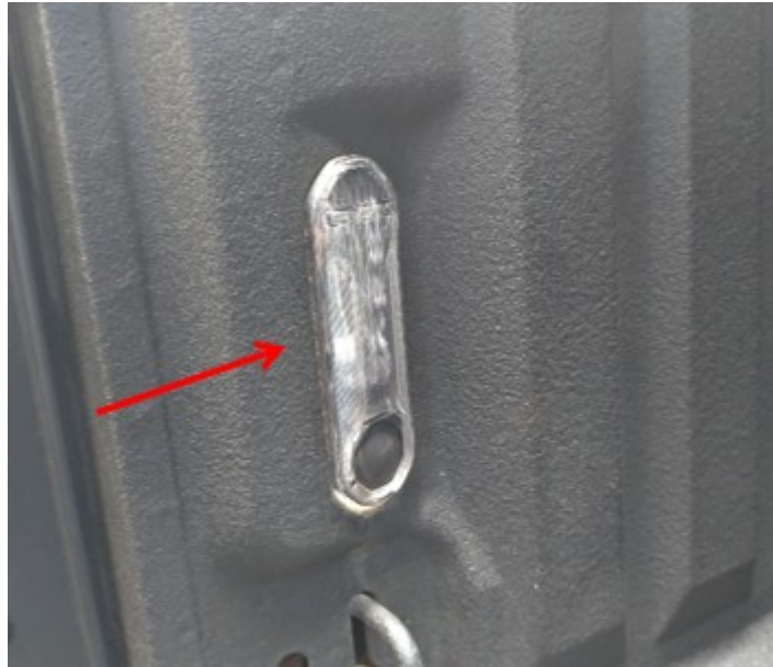
Fig. 3 Pickup Box Light Installed
