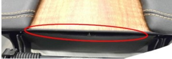
Fig. 1 Console Lower Cover Separating
