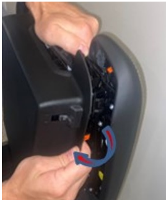
Fig. 3 Lower Cover From Pawls
