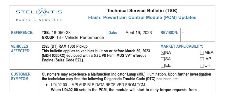
Transmission Control Module (TCM), the transmission will fault and go to a fixed gear limp-in
