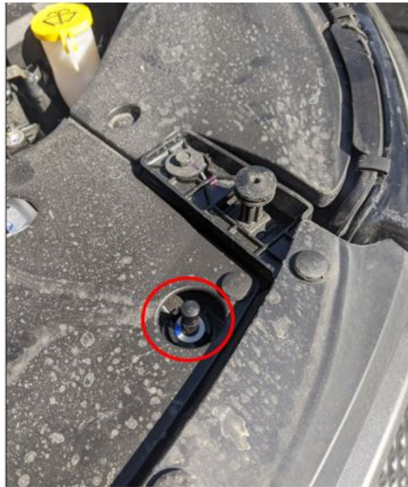
Fig. 1 Hood Switch Location
