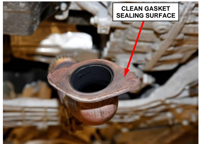
Figure 29 – Crossunder Pipe Flange
