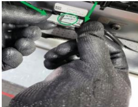
Fig 2 Connector fully “push, click, push, push” seated.
