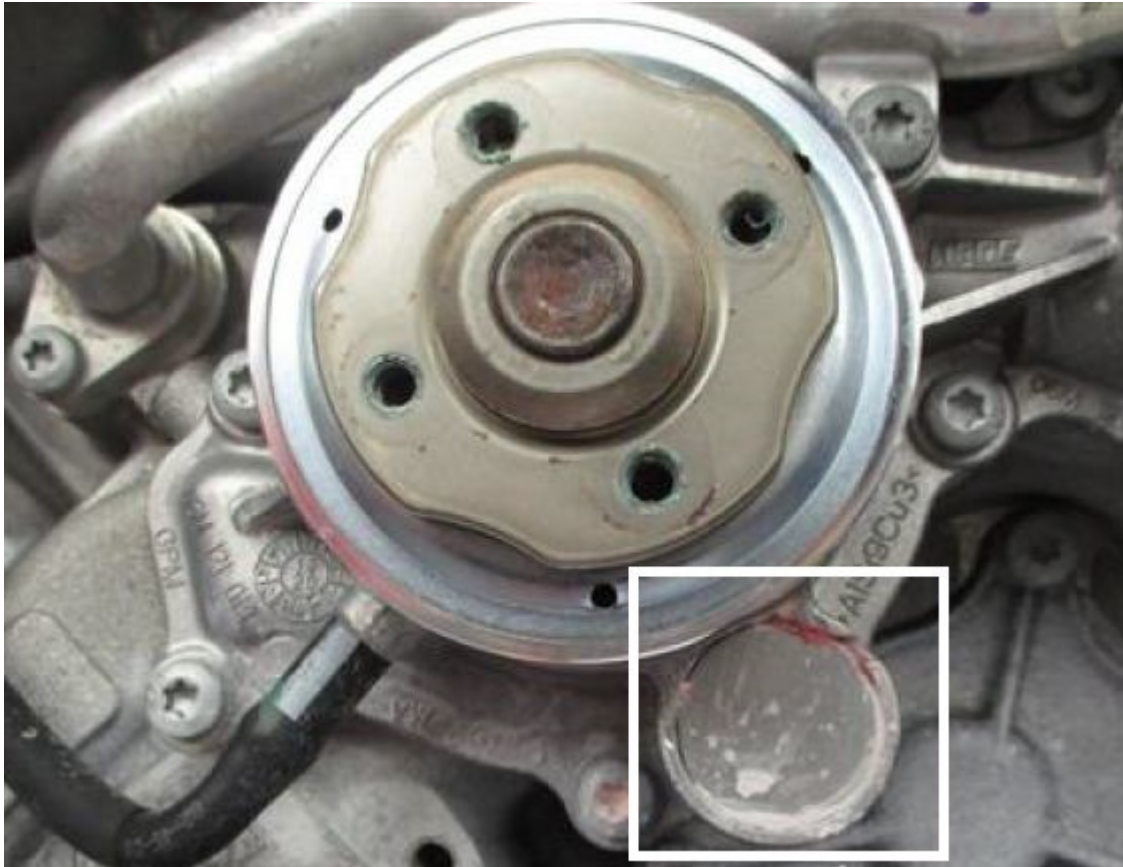
Figure 1: Traces of coolant on the drip cup.
