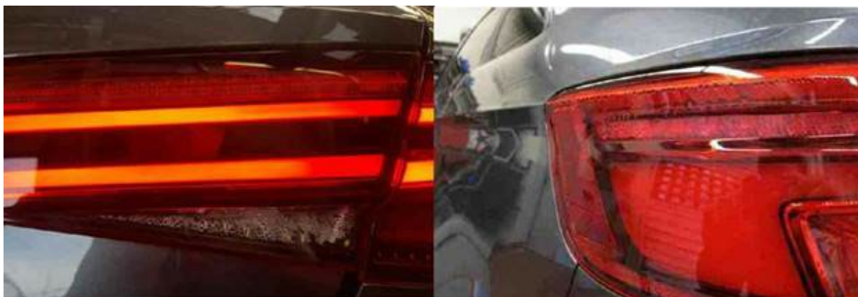
Figure 4: Example of compromised tail lamps after a sufficient test drive.
