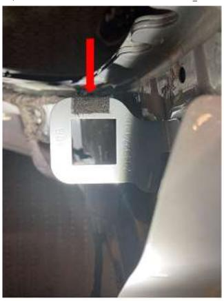
Apply felt tape to the upper edge of the square eye of the body support bracket (*photo shows a bare body shell for clarity*).
