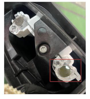
2. Inspect the headlamp and LED module for signs of discoloration as shown in the photo.
