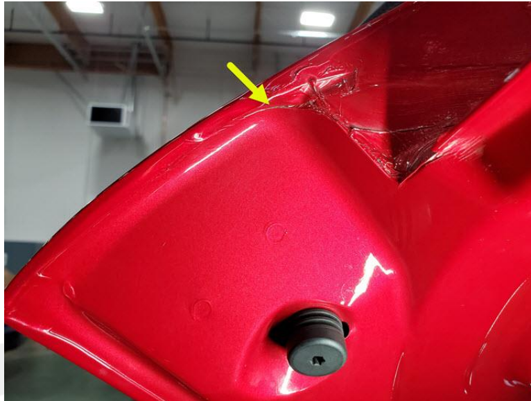
Figure 26 – Example of trunk lid seam
