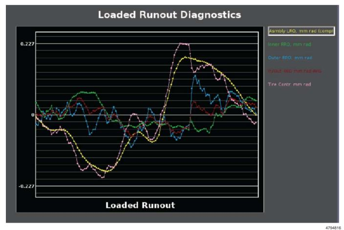
The Hunter Road Force Balancer allows technicians to review the Road Force Data and Plots that were measured. This allows technicians to determine the high and low spots on the tire. These should be used for a visual inspection when looking for defects or signs of road hazard damage.
