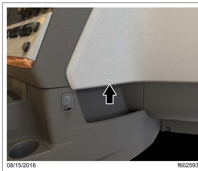
Fig. 8, Electrical Bay Cover Location
