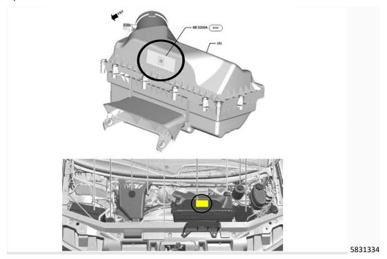
2. Clean the label area on the airbox using a non-oil based cleaner, preferably isopropyl alcohol (rubbing alcohol), Kent Acrysol, P/N 20005, or an equivalent cleaning solvent.
